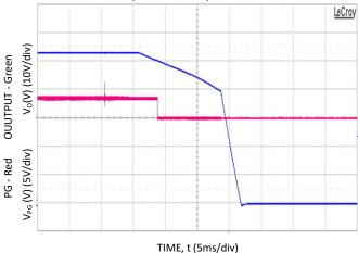
Figure 12. PG# alarmed 10ms prior to Vo < 40V,  $V_{IN}$  = 230V<sub>AC</sub>, Output at Full load
