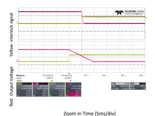
Figure 17: Time delay from interlock reverse and output shut down. interlock signal can be used as quick turn off signal.
