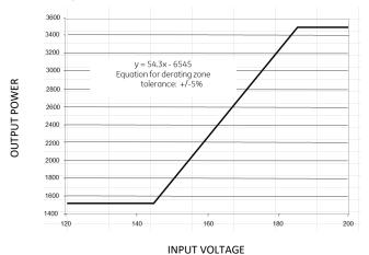
Figure 18. Output power derating below V<sub>IN</sub> of 185V<sub>AC</sub>
