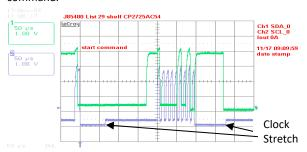
Figure 15. Example waveforms showing clock stretching.
