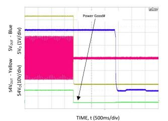
Figure 15. Turn-OFF at full load,  $V_{\text{IN}}$ =230 $V_{\text{AC}}$
