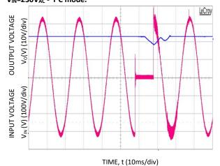
Figure 11. Ride through missing ½ cycle, full load,  $V_{\text{IN}}$  = 230 $V_{\text{AC}}$ .
