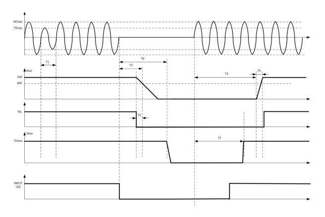
T1 - ride through time - 0.5 to 1 cycles [ 10 - 20ms]  $V_{OUT}$  remains within regulation - load dependent
