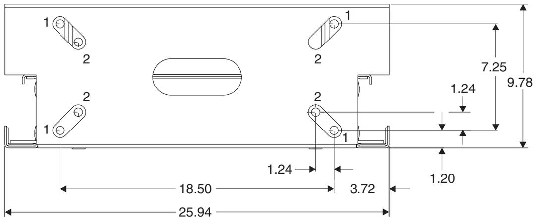
If interference with floor reinforcing bars occurs during installation of anchoring hardware at mounting position "1" (primary mounting positions), use position "2" alternate mounting positions.
