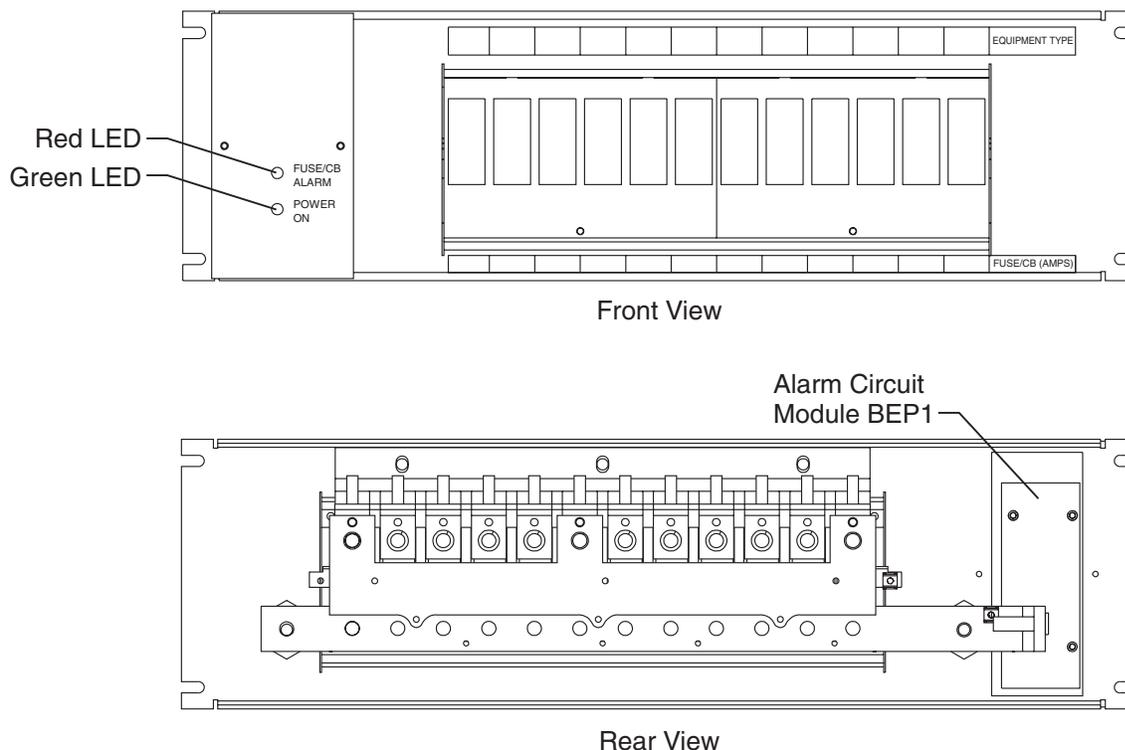
Figure 5-4B: List D Circuit Breaker Panel for J85568E-1 Mini-Distribution Bay
