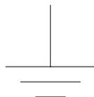
This symbol is used to identify other bonding points within the equipment.
