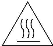
This symbol is used to identify the presence of a hot surface. The marked item should not be touched without taking care.
