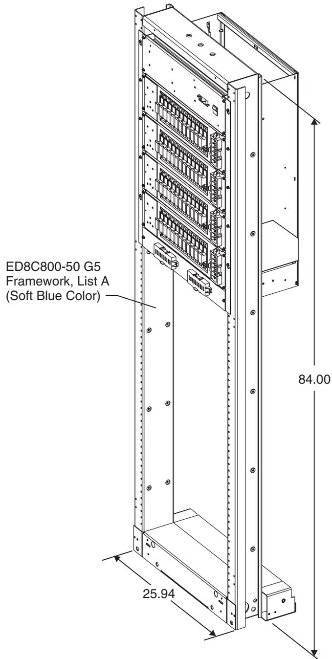
**Figure 2-2: J85568E-1 Mini-Distribution Bay Factory Installed in ED8C800-50 G5 Framework (four fuse panels shown)**
