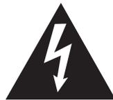
This symbol is used to identify the presence of hazardous ac or dc voltages. It may also be used to warn of hazardous energy levels.
