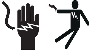
These symbols (or equivalent) are used to identify the presence of hazardous ac mains voltage.
