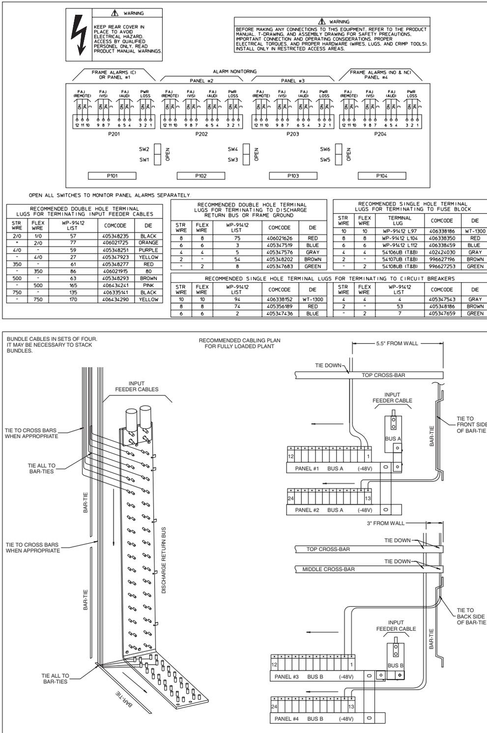
Figure 5-7: Installation Information Label (Rear of Mini-Distribution Bay)
