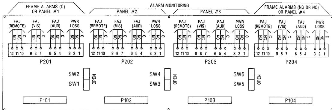
**Figure 5-6: Alarm Termination Board**
