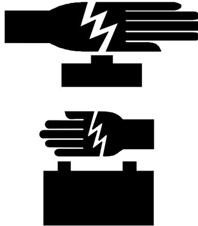
One of these two symbols (or equivalent) may be used to identify the presence of rectifier and battery voltages. The symbol may sometimes be accompanied by some type of statement, for example: “Battery voltage present. Risk of injury due to high current. Avoid contacting conductors with uninsulated metal objects. Follow safety precautions.”
