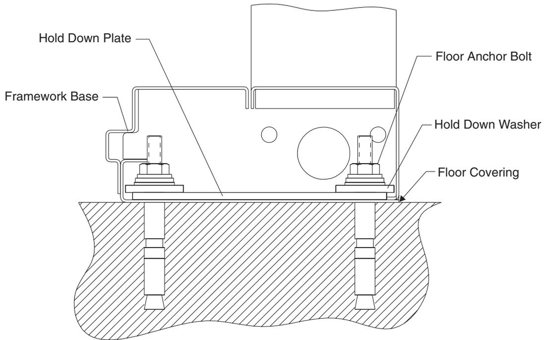
Note: Use 3/4 Inch Drill for Floor Anchor Bolts.
