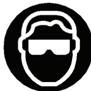
This symbol is used to identify the need for safety glasses and may sometimes be accompanied by some type of statement, for example: “Fuses can cause arcing and sparks. Risk of eye injury. Always wear safety glasses.”
