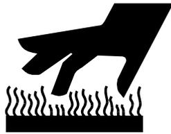
This symbol is used to identify the presence of a hot surface. It may also be accompanied by a statement explaining the hazard. A symbol like this with a lightning bolt through the hand also means that the part is or could be at hazardous voltage levels.
