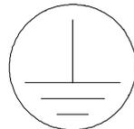
This symbol is used to identify the protective safety earth ground for the equipment.
