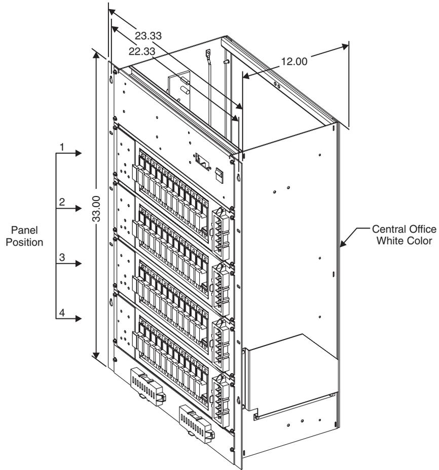
**Figure 2-1: J85568E-1 Mini-Distribution Bay (four fuse panels shown)**
