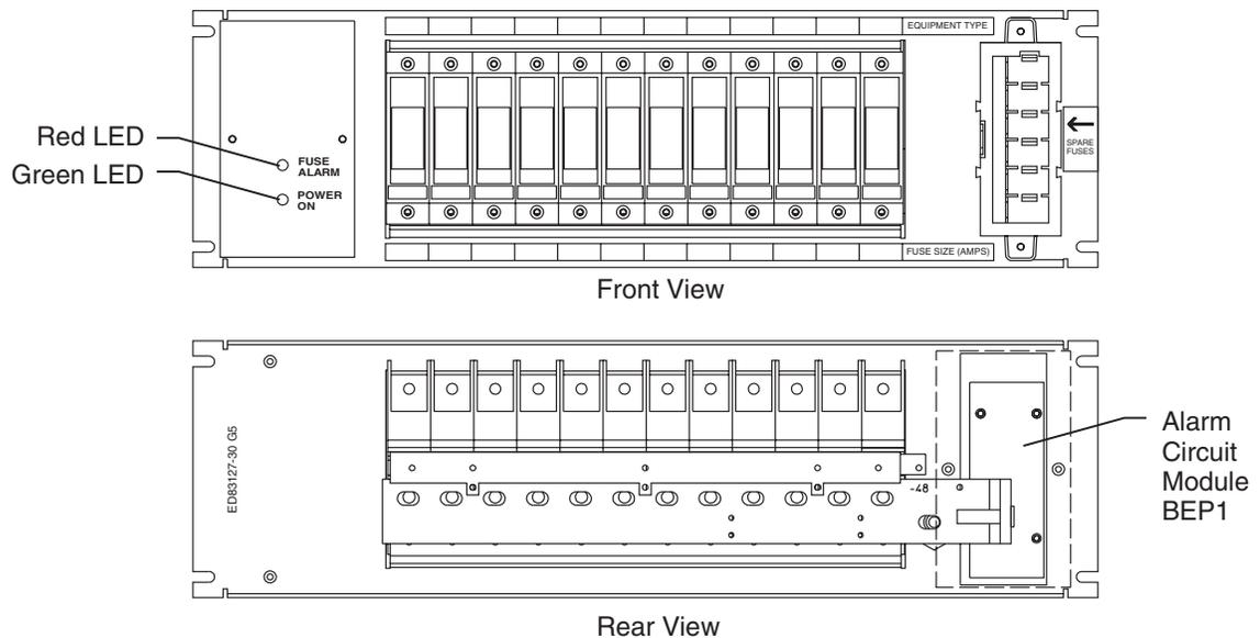
**Figure 5-4A: List C Fuse Panel for J85568E-1 Mini-Distribution Bay**
