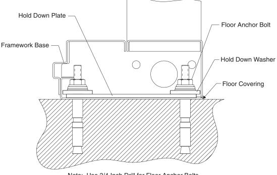
Note: Use 3/4 Inch Drill for Floor Anchor Bolts. The Required Minimum Drill Depth is 4 Inches.
