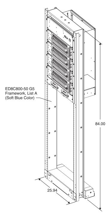
Figure 2-2: J85568E-1 Mini-Distribution Bay Factory Installed in ED8C800-50 G5 Framework (four fuse panels shown)
