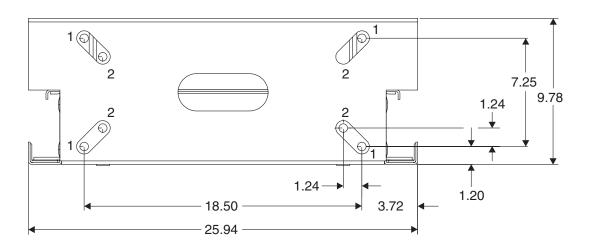
If interference with floor reinforcing bars occurs during installation of anchoring hardware at mounting position "1" (primary mounting positions), use position "2" alternate mounting positions.
