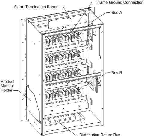
Figure 5-3: Rear View of Mini-Distribution Bay and A/B Load Connections (four fuse panels shown)
