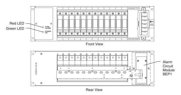
Figure 5-4A: List C Fuse Panel for J85568E-1 Mini-Distribution Bay
