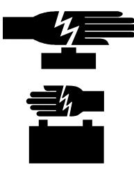
One of these two symbols (or equivalent) may be used to identify the presence of rectifier and battery voltages. The symbol may sometimes be accompanied by some type of statement, for example: "Battery voltage present. Risk of injury due to high current. Avoid contacting conductors with uninsulated metal objects. Follow safety precautions."
