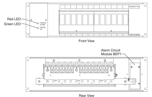
Figure 5-4B: List D Circuit Breaker Panel for J85568E-1 Mini-Distribution Bay
