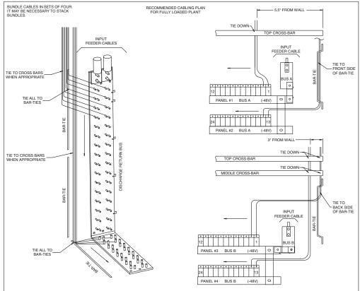
Figure 5-7: Installation Information Label (Rear of Mini-Distribution Bay)
