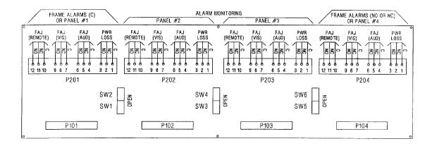
Figure 5-6: Alarm Termination Board
