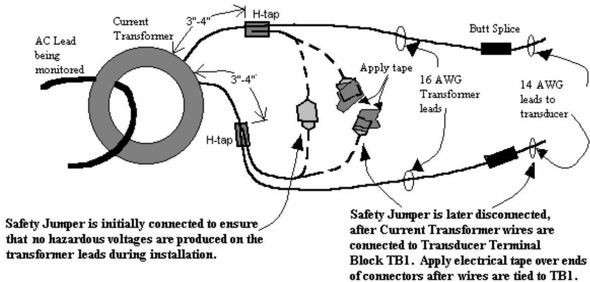
Figure 4. Use of Safety Jumpers (Rev. B and later units)
