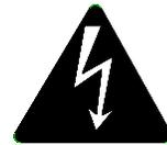
This symbol is used to identify the presence of hazardous AC or DC voltages. It may also be used to warn of hazardous energy levels.
