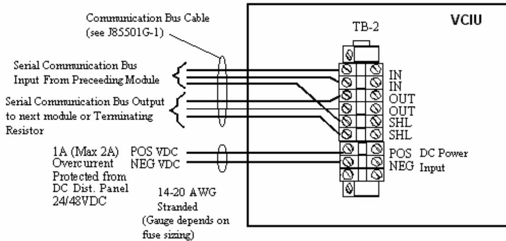
Figure 5 - Galaxy communications network and DC Power wiring
