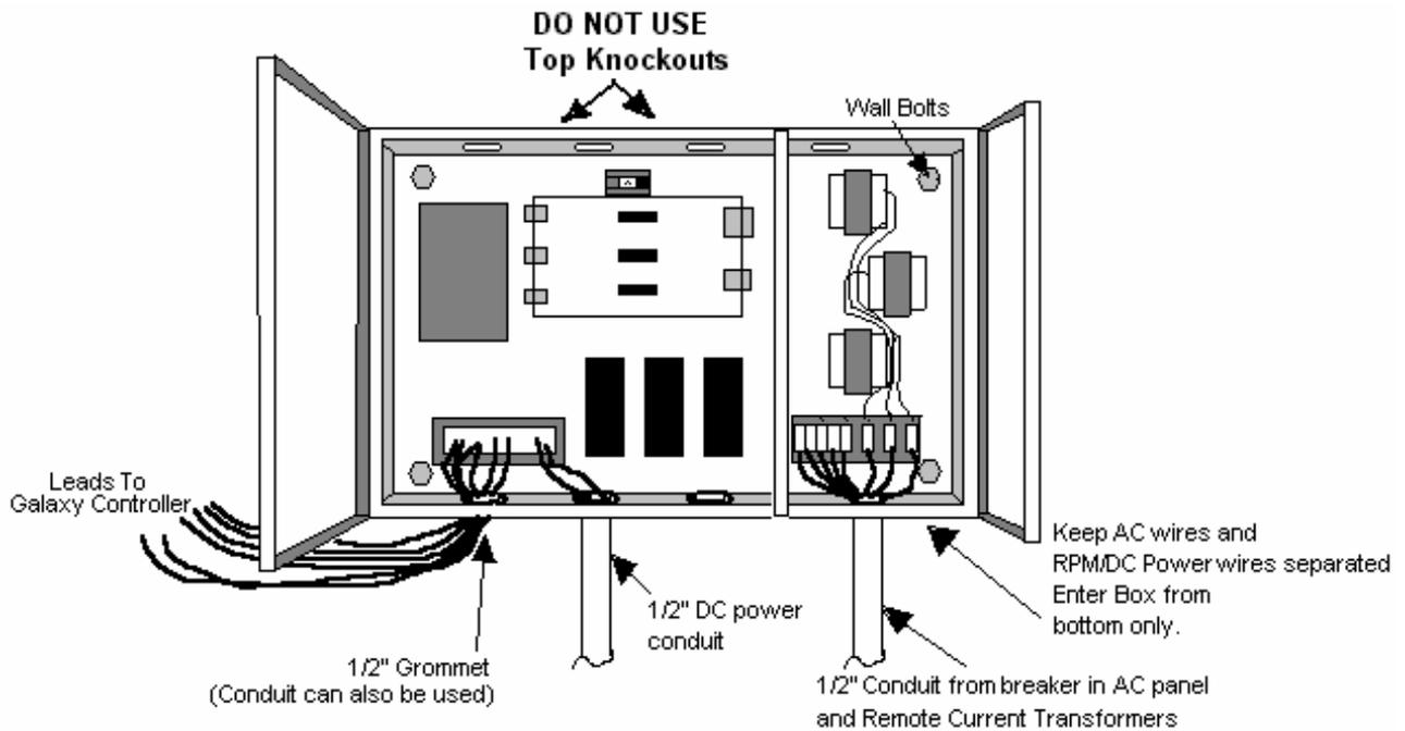
**Figure 1 – Conduit and Wire Routing, Typical**
