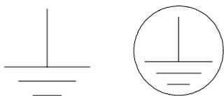
The above symbols (or the “GND” symbol) are used to identify the safety earth ground or bonding point for the equipment.
