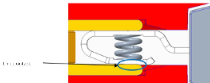
ReliaGear neXT and SB finger assembly, showing line contact area
