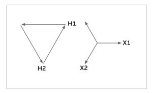
We have a requirement to feed a four-floor data center. Each two-floor space has the same quantity and type of computers working at the same time. We will feed one two-floor space with 0° Guard III transformers and the second two-floor space with a 30° Guard III transformer. The harmonics profile of each transformer load per unit is as follows:
