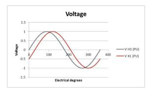
Two sinusoidal waves have different phases when their peaks do not occur at the same time. The difference in electrical degrees is the phase angle between them. Some transformer connections can induce a phase shift in current. For example, a Delta–Y connection induces a 30° phase shift between the primary and secondary side of the transformer.
