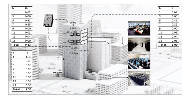
The key to achieve this cancelation is balance. Non-linear loads should be distributed to reach an optimum balance in the phases and the transformers involved in the cancelation. Capacity is not the only important factor. The type of load must be considered. Each electronic load has a particular harmonics profile and is required to reach the maximum cancelation effect in the same harmonic profile in each phase of the transformers.
