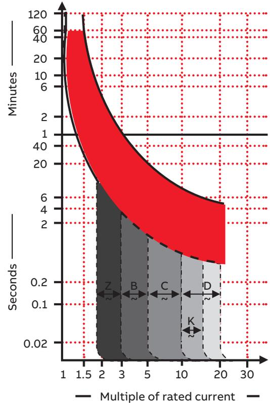
Understanding trip curves and being able to identify the differences among them based on the MCB functionality will facilitate the selection of the right trip curve. Selecting the correct trip curve for an MCB can potentially enhance the protection and lifetime of connected loads.
