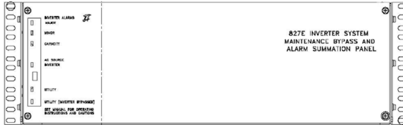
FIGURE 2-1: Front View of the 6310408P 10KVA Bypass Panel
