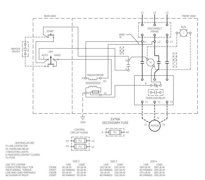
NOTE: ADDITIONAL OVER-CURRENT PROTECTION MAY BE REQUIRED. REFER TO THE NATIONAL ELECTRICAL CODE OR LOCAL ELECTRICAL CODE AS REQUIRED.
