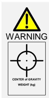
**WARNING:** AN OUT OF BALANCE CONDITION COULD OCCUR. THE MBC CABINET IS HEAVY AND TALL, THEREFORE, THE CENTER OF GRAVITY (COG) MAY NOT BE IN AN OBVIOUS LOCATION. TILTING A UNIT MORE THAN 10 DEGREES CAN CAUSE A HAZARDOUS SITUATION.
