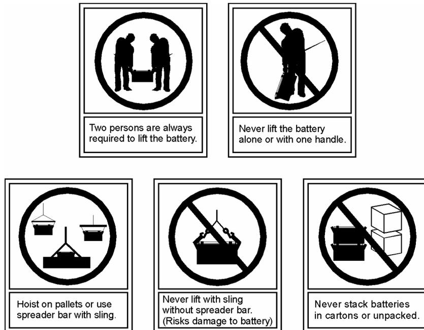
Figure 5-3: Battery Lifting Precautions
