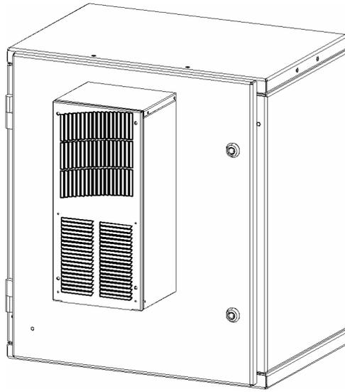
**Figure 2-3: G19 with protruding Air Conditioner – Front View**
