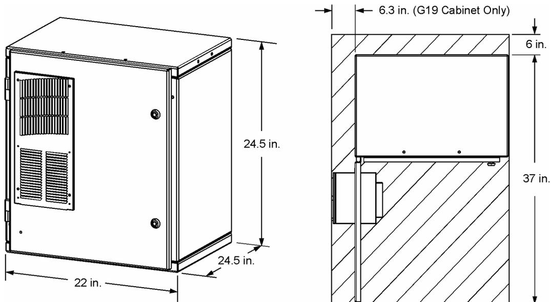
Figure 4-1: G18/G19 Cabinet Dimensions and Clearances
