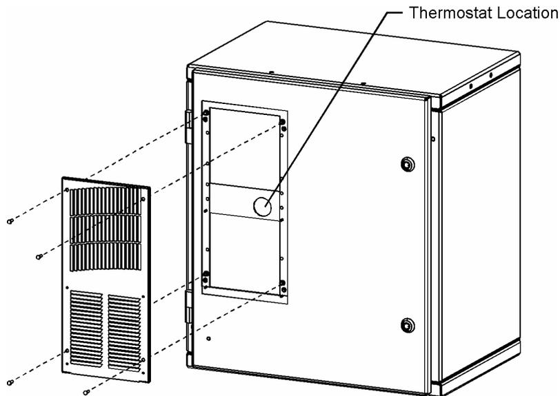
Figure 7-2: Air Conditioner Thermostat Location
