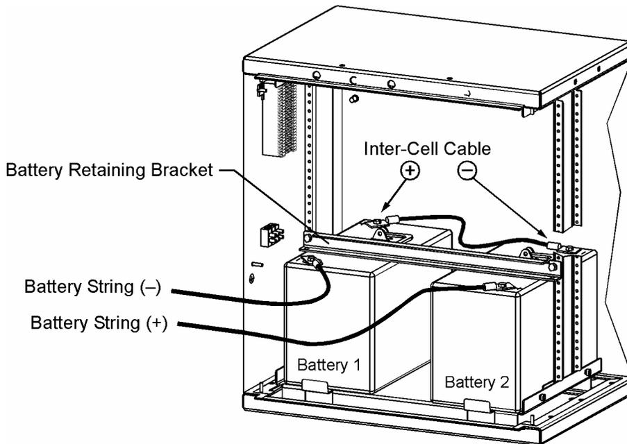
3. Remove any terminal covers from each of the battery modules and spread a thin coat of antioxidant on all of the battery terminals.
