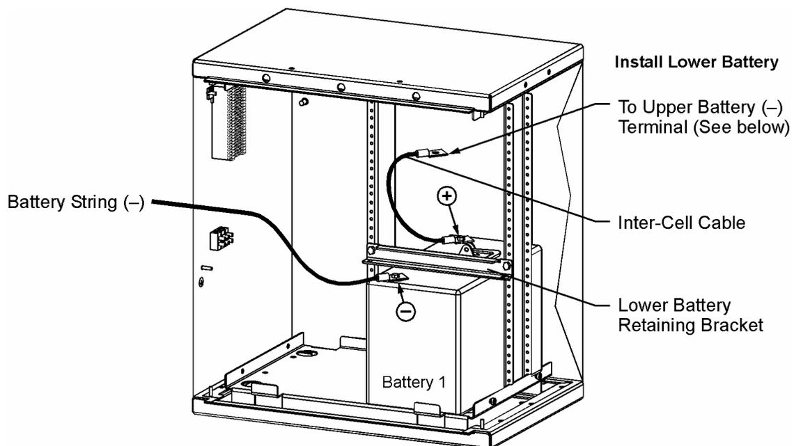
3. Remove any terminal covers from the battery module and spread a thin coat of antioxidant on the battery terminals.
