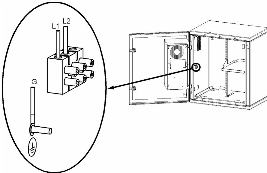
Figure 4-3: Air-conditioner AC Power input
