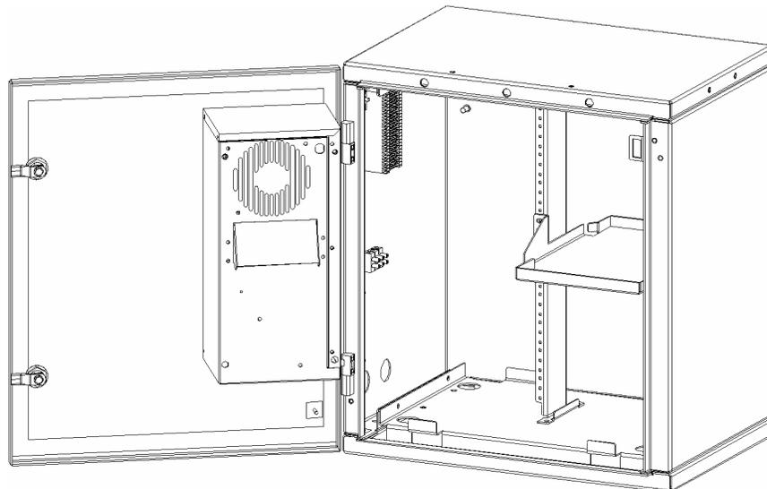
**Figure 2-2: G18 with Recessed Air Conditioner – Internal View**
