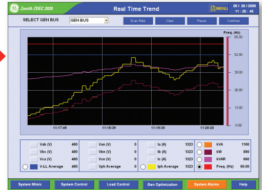
Generator Bus Trend Screen
