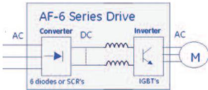
All GE AF-6 series drives come standard with a DC link reactor and can have additional line impedance added for further mitigation. They are available in NEMA 1, 12 and 3R enclosures and with ratings up to 300 horsepower. For more details and product selection, see the Control Catalog (GEP-1260P) or Standard Drives Buyers Guide (GEP-S1000E).
