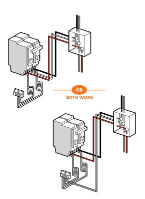
In retrofit applications, most AFCIs require a clean neutral return to the circuit breaker to prevent nuisance tripping. In these situations, there is a high probability that neutral wires are tied together throughout the house. Searching out all of these wire runs is both cumbersome and time-intensive.
