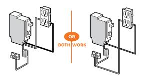
Unlike other brands, the neutral load lug on the GE AFCI breaker is there simply for your wiring convenience. For new construction you have the option to run the neutral wire back to the breaker or the ground bar. For retrofits it's a true time-saver. You don't have to track down the exact neutral wire that may be split or shared upstream- you can simply pull and replace.
