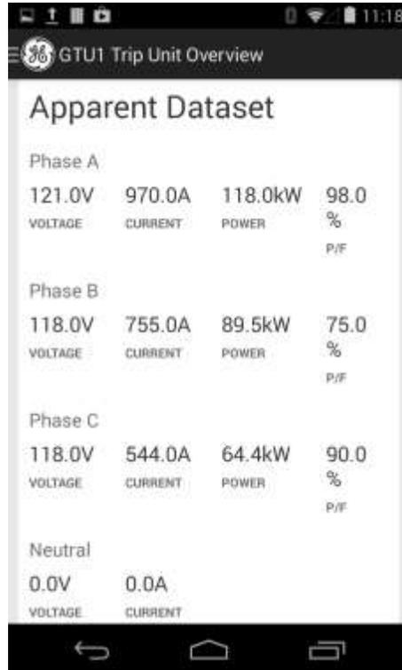
Figure 10. Trip Unit Overview Monitoring Breaker
