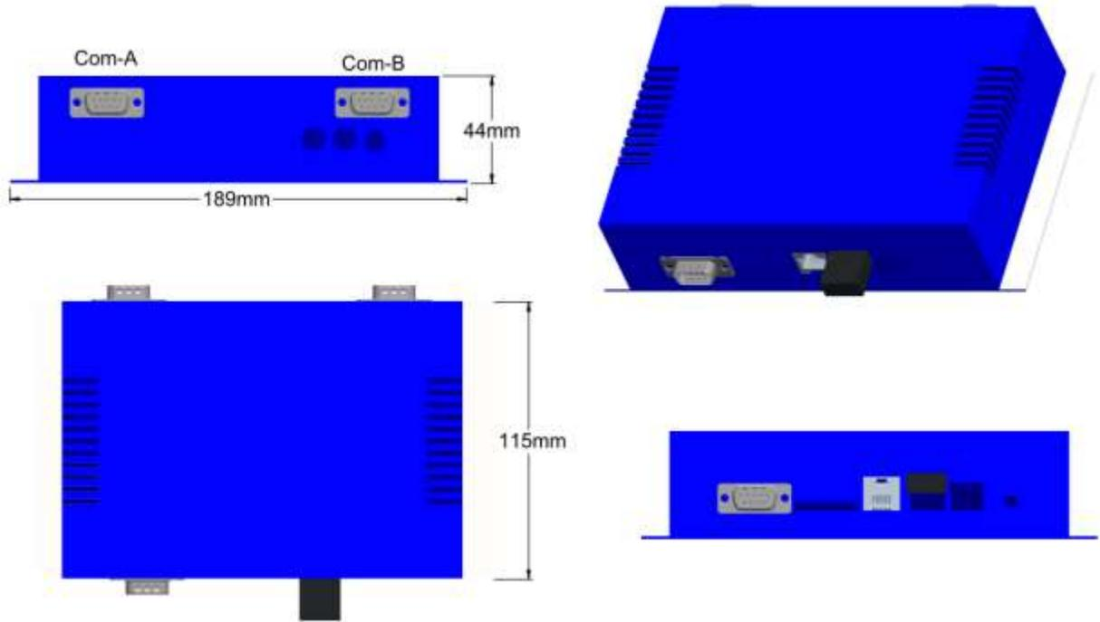
Figure 2. Hardware Dimensions (mm) and Appearances
