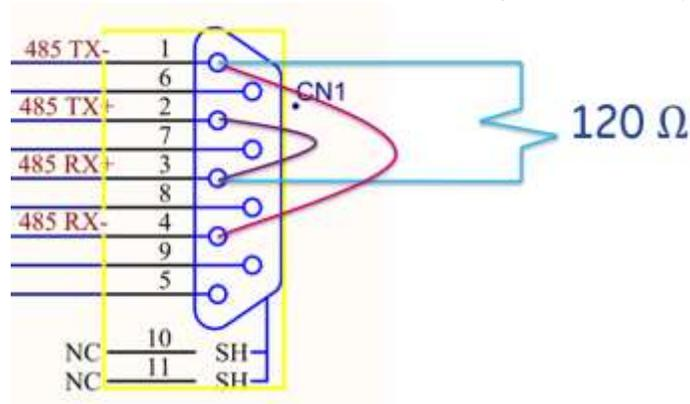
Figure 3. Wiring DB9 Connector
