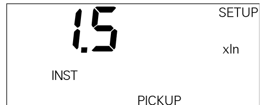
Figure 16. Trip Unit display for instantaneous pickup.
