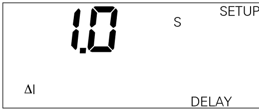
Figure 26. Trip Unit display for current-unbalance relay delay.
