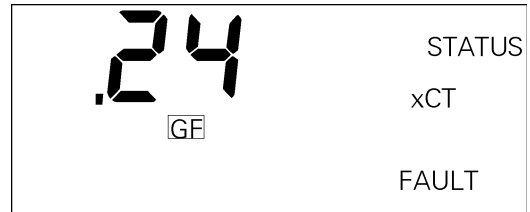
Figure 56. Trip Unit status display for ground-fault trip.
