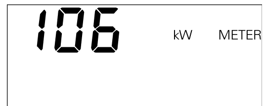
Figure 46. Trip Unit display for aggregate real power.
