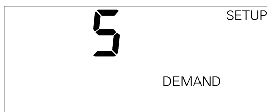
Figure 39. Trip Unit display for power demand interval.
