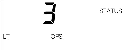
Figure 58. Trip Unit status display for long-time overcurrent trip counter.
