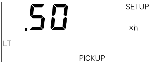
Figure 7. Trip Unit display for long-time pickup.
