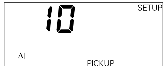
Figure 25. Trip Unit display for current-unbalance relay pickup.
