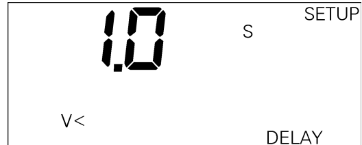
Figure 30. Trip Unit display for undervoltage relay delay.
