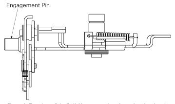
Figure 3. Top view of the Bell Alarm mounting plate, showing the pin to engage the breaker mechanism.
