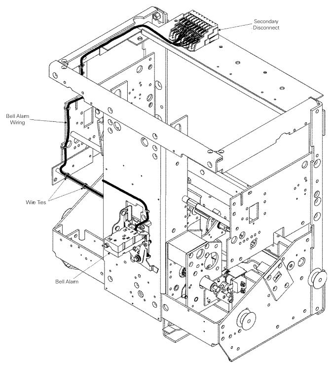
Figure 5. Path for routing wires from the Bell Alarm with Lockout to the secondary disconnect.
