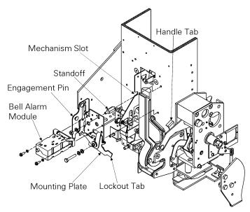
Figure 2. Installation of the Bell Alarm with Lockout.
