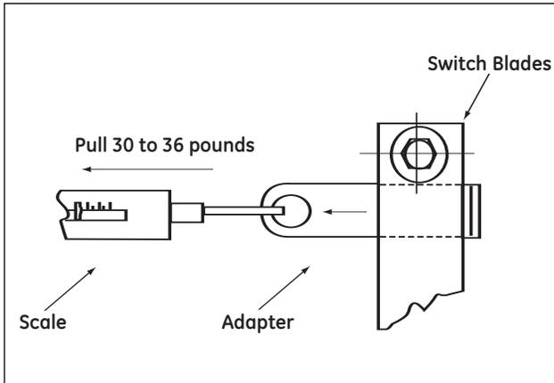
**Step 5: Jaw Contact Pressure Adjustment**
