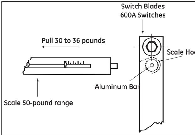
**Step 4: Hinge Contact Pressure Adjustment**
