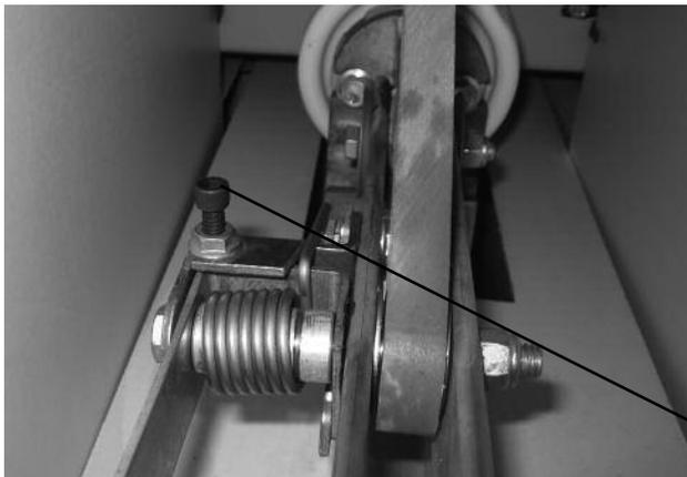
If any corrections in the arcing blade position are necessary (after all previous steps have been completed), loosen the locknut on the arcing blade adjusting screw – see Figure 10 – and turn the screw either in or out to obtain positioning of arcing blade. Re-tighten the locknut.
