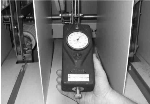
A force of 2-4 pounds should be necessary to move the blades. Loosen or tighten the hinge bolt as necessary to meet the 2-4 pound requirement.
