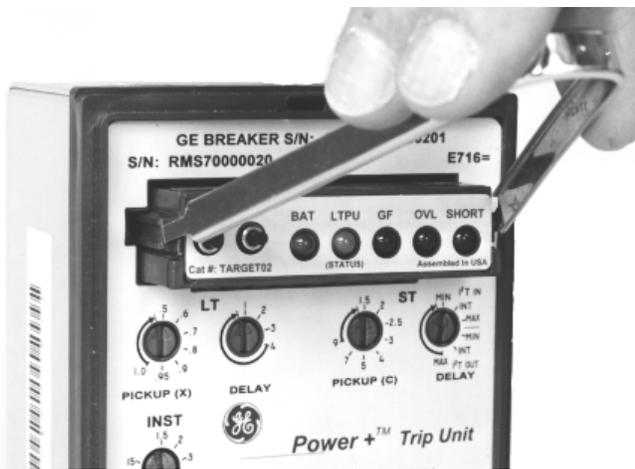
Figure 7. Removing the target module (a Power+ Trip Unit is shown).
