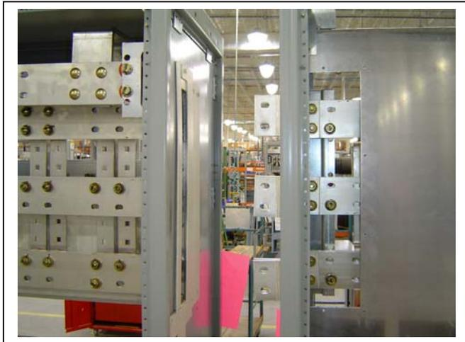
Use a screwdriver to make sure the holes align. Then add the hardware to join the bus and splice bars.
