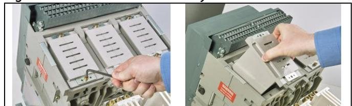
2. Insert the wear indicator in each pole as shown in Fig 8.3.
