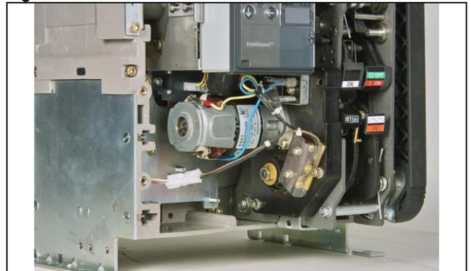
5. Use an M8 nylock nut to mount the motor switch actuator onto the shaft end, torque to 14.5 N m.
