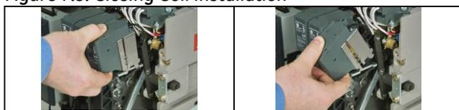
Connect the wire plugs (Fig. 7.6) according to the wiring schematic in Section 3.
