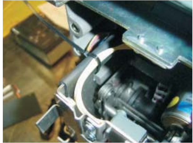
Figure 4. Assembling wire tie
