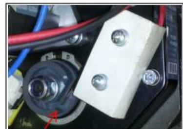
Figure 6. Cam Orientation when charged
