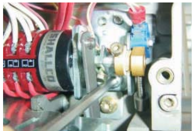
Figure 4. Remove the Screw & nut
