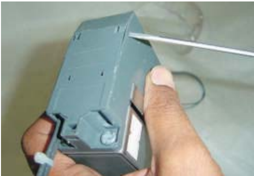
Figure 2. Removing the existing cover
