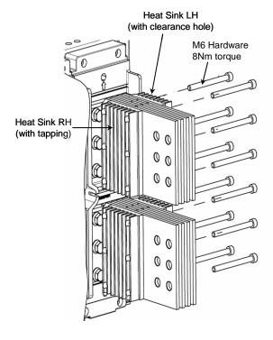
Fig B. Heat sink assembly to terminal assembly for 3000 Amperes (UL)
