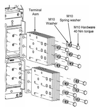
Fig A. Back Connected Terminations assembly for 3000 Amperes (UL)
