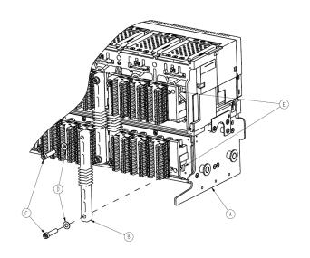
Fig C. Envelope 3-200kA Cluster pad support assembly
