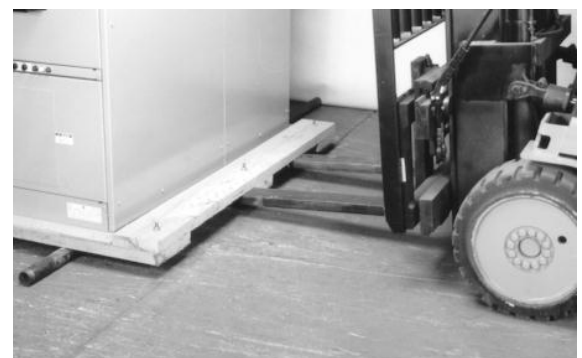
— Fig. 2.7 Placement of rollers under shipping skid
