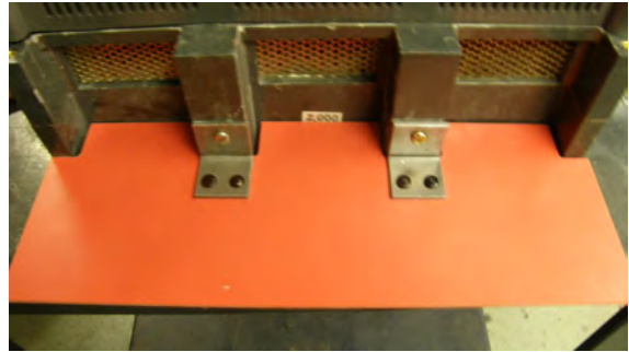
Figure 6: Line Shield Installation
