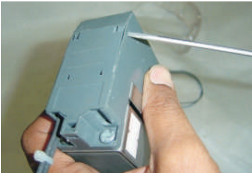
Figure 2. Removing the existing cover
