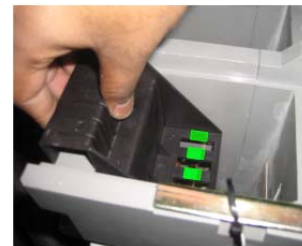
Figure 8.3. Wear Indicator Insertion
