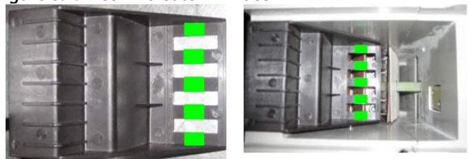
Figure 8.4. Wear Indicator in Place
