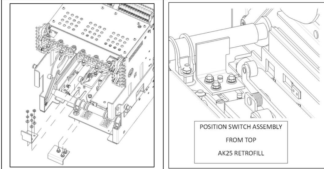
3. Insert the 3-pin bracket from the bottom of the base of the cassette assembly, such that the two pins are within the longer slot and the single pin goes inside the smaller slot of the plate.
