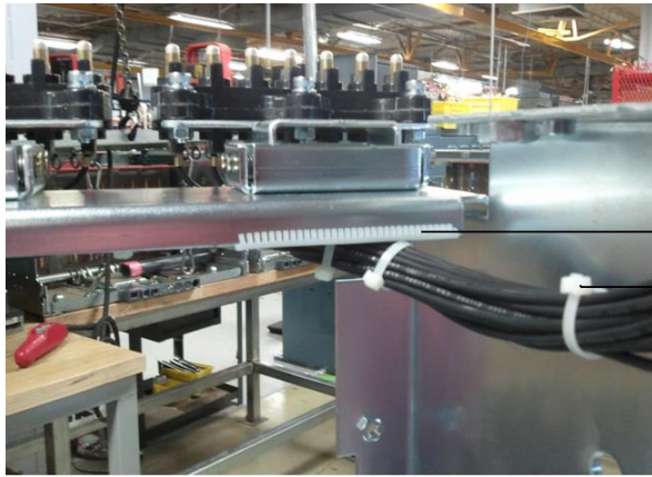
Figure 49. Wires from Secondary Bullets
