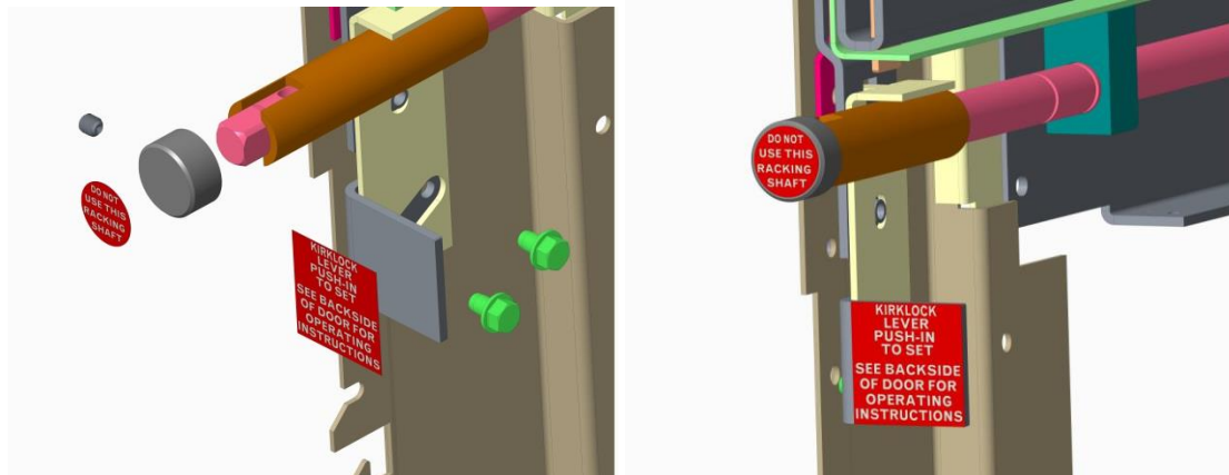
Figure 10A / 10B. AK-50 & AKT-50 – Retrofill Kits
