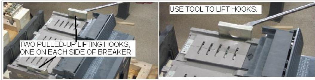
Figure 7. AKD-5—Breaker Lifting Holes
