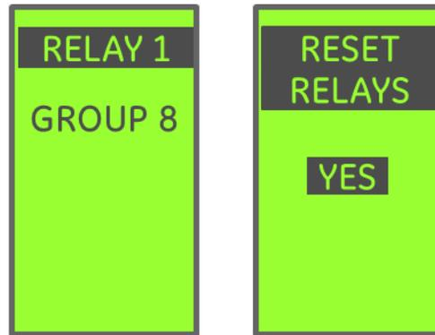
Output Relay configuration **Group 8** (ALARM and TRIP) links the relay to the GF Sum Alarm, GF Sum Trip, GF CT Alarm, and GF CT Trip protection functions.
