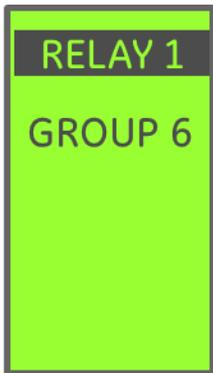
Output Relay Configuration **Group 6** links the output relay to the Error status of the trip unit. Any internal error condition that results in a display on the Error Status screen will set this output. The output does not latch – it remains energized as long as the error condition persists.
