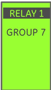
Output Relay configuration **Group 7** links the relay to the Reduced Energy Let Through (RELT) function. Whenever RELT is engaged the output relay will be closed.
