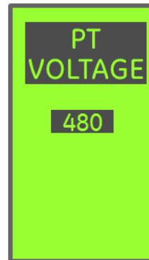
**PT Voltage** configures the trip unit so that a full scale reading at the potential transformer input is correctly scaled.
