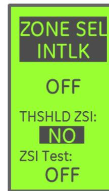
**Threshold ZSI** is a specialized function. It is only available when the I-ZSI option is installed in the trip unit. When active, a downstream breaker will command its ZSI Output signal ON when the affected element reaches 80% of pickup. When an upstream breaker has Threshold ZSI enabled and it receives a ZSI input from a downstream breaker it will increase its ZSI pickup setpoint to 123% of the user setpoint.
