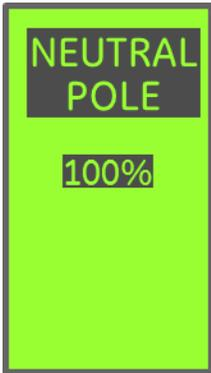
**Neutral Pole** setting determines the overcurrent protection setting for the neutral pole of a 4 pole breaker.
