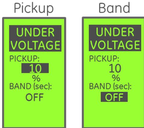
**Undervoltage** is part of the optional protective relay feature. If protective relaying is not installed on the trip unit, this screen will not appear.
