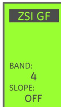
The **Zone Selective Interlock (ZSI) GF** setting sets an alternative GF delay band and slope setpoint combination that will override the GTU GF setpoints whenever the trip unit receives a valid ZSI input signal.
