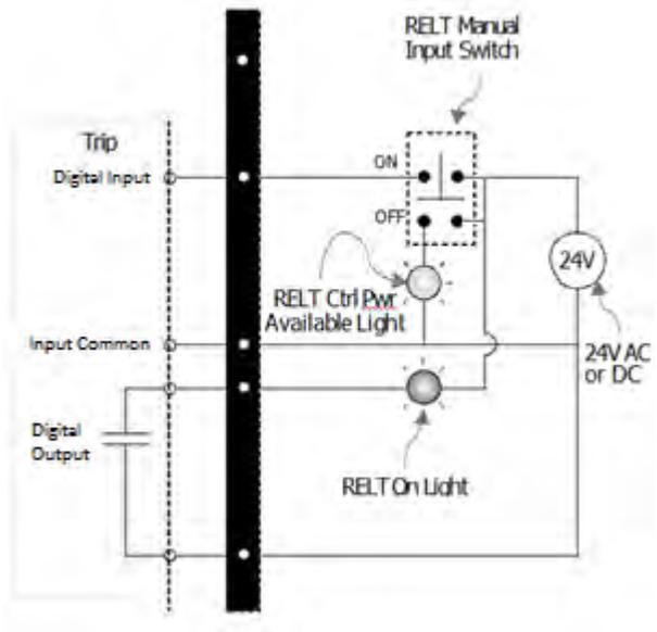
Figure 10-2: RELT Connection without Positive Feedback from EntelliGuard TU Trip Unit
