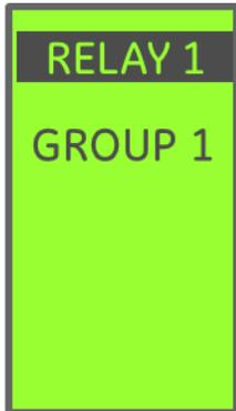
Output Relay configuration **Group 1** links the Output Relay to the GF Sum Alarm and GF CT Alarm protection functions.
