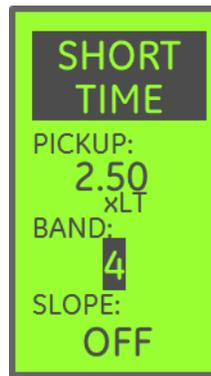
The **Short Time** element protects the electrical system from higher level overloads and moderate short circuit currents.
