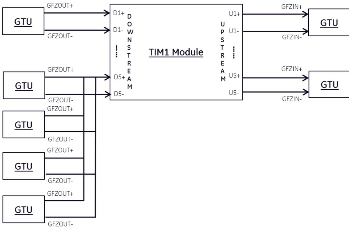
A **maximum of six** trip units can be connected in parallel to a **single DOWNSTREAM TIM1 input pair**.
