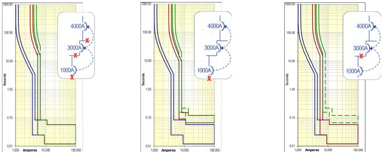
All breakers set for maximum protection. 3000A and 4000A breakers overlap.
