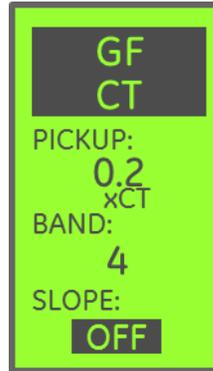
**Ground Fault CT Slope** modifies the shape of the “delay band” for the GF element.
