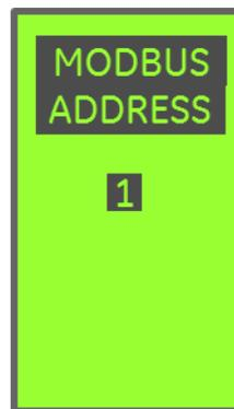
Sets the Modbus communication parameters for the trip unit.
