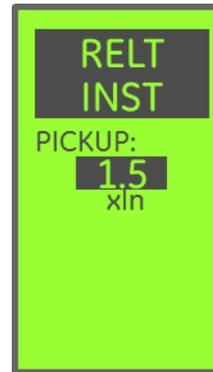
**Reduced Energy Let-Thru (RELT)** is a second Instantaneous protection element that is fully independent of all other protection elements. RELT can be engaged or disengaged by dedicated remote contact or via communications. It cannot be controlled from the local keypad on the trip unit.
