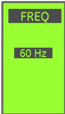
Frequency sets the trip unit's internal frequency to match the system frequency.
