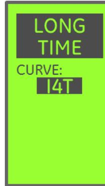
**Long Time Curve** selects the type of LT protection curves available for configuration.
