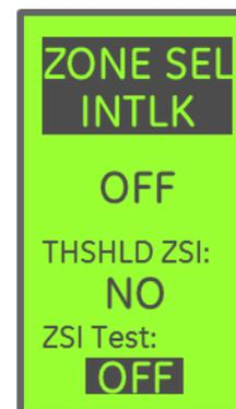
The **ZSI Test Setup** screen provides a useful diagnostic tool for setting up or periodically evaluating your ZSI network. If ZSI Test is set to ON the trip unit will command its ZSI Output signal to be ON for 30 seconds. After 30 seconds has elapsed the ZSI output will be automatically turned off.
