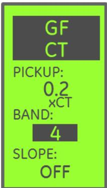
**Ground Fault CT Band** selects the “delay band” for the GF element, or how long the trip unit will allow an overload to persist before the breaker is commanded to open.
