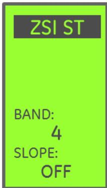
The **Zone Selective Interlock (ZSI) ST** setting is an alternative ST delay band and slope combination that will override the GTU ST setpoints whenever the trip unit receives a valid ZSI input signal. This equates to the RESTRAINED, selective setting.
