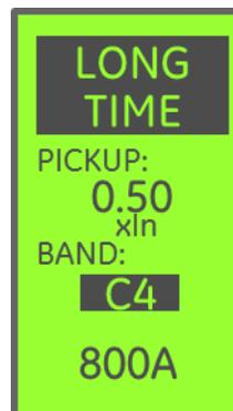
**Long Time Band** selects the "delay band" for the LT element, or how long the trip unit will allow an overload to persist before the breaker is commanded to open.
