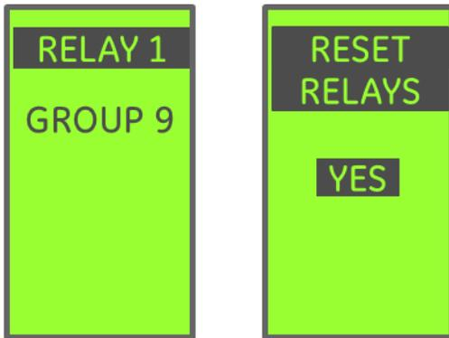
Output Relay configuration **Groups 9, 10, and 11** (IEC devices only) link the relay to the REF Trip, SEF Trip, and UEF Earth Fault Trip protection functions, respectively.
