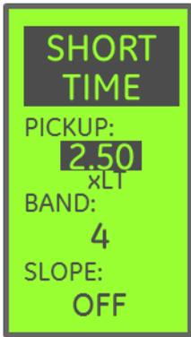
**Short Time Pickup** defines the threshold where the ST element begins to “timeout” toward tripping, as a multiple of the Long Time Pickup threshold.
