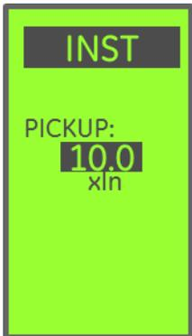
**Instantaneous Pickup** defines the threshold where the INST element begins to “timeout” toward tripping, as a multiple of the Rating Plug current (In).
