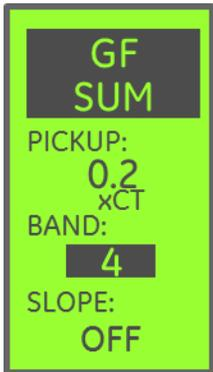
**Ground Fault Sum Band** selects the "delay band" for the GF element, or how long the trip unit will allow an overload to persist before the breaker is commanded to open.
