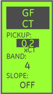
The **Ground Fault CT** element protects the electrical system against unintentional connections to earth ground.
