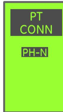
**PT connection** allows the trip unit voltage input configuration to be set to match the wiring of incoming Potential Transformer (PT).
