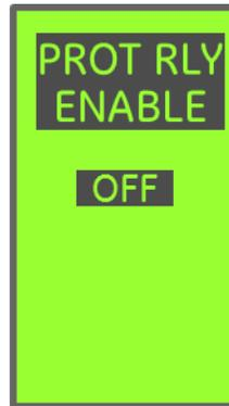
The **Protective Relay** setting screen enables or disables tripping for protective relays:
