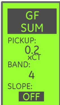
**Ground Fault Slope** modifies the shape of the "delay band" for the GF element.
