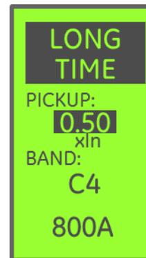
**Long Time Pickup** defines the fault current threshold where the Long Time protection element begins to "timeout" toward tripping as a percentage of the Rating Plug current (In). The actual pickup threshold, in amperes, is indicated at the bottom of the screen
