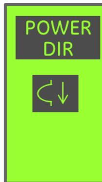
**Power Direction** describes to the trip unit how power is flowing through the breaker, and thus determines the polarity.
