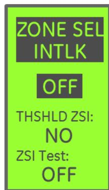
The optional **Zone Selective Interlocking (ZSI)** feature allows enhanced coordination of tiered breaker installations.
