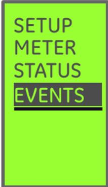
The EntelliGuard Trip Unit maintains up to 10 event records. These records can be accessed from the front panel by selecting the EVENT menu item and scrolling through the available event records. The EntelliGuard Setup Software will also allow event retrieval and viewing via serial communications.
