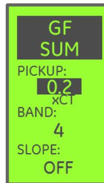
The **Ground Fault Sum** element protects the electrical system against unintentional connections to earth ground.
