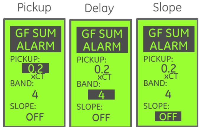
This is the **Ground Fault Sum Alarm Setup Screen**.
