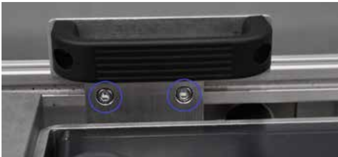
Figure 4-3: Slide Assembly Mount Bolts, A&B
