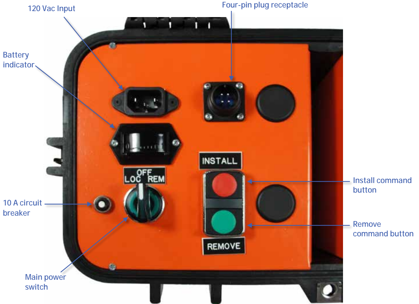
Figure 5-2: RSO Control Panel Components
