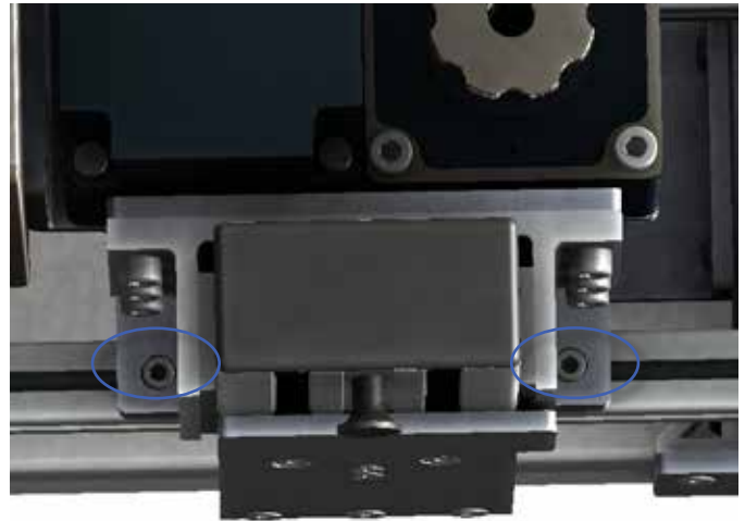
Figure 4-4: Slide Assembly Mount Bolts, C&D
