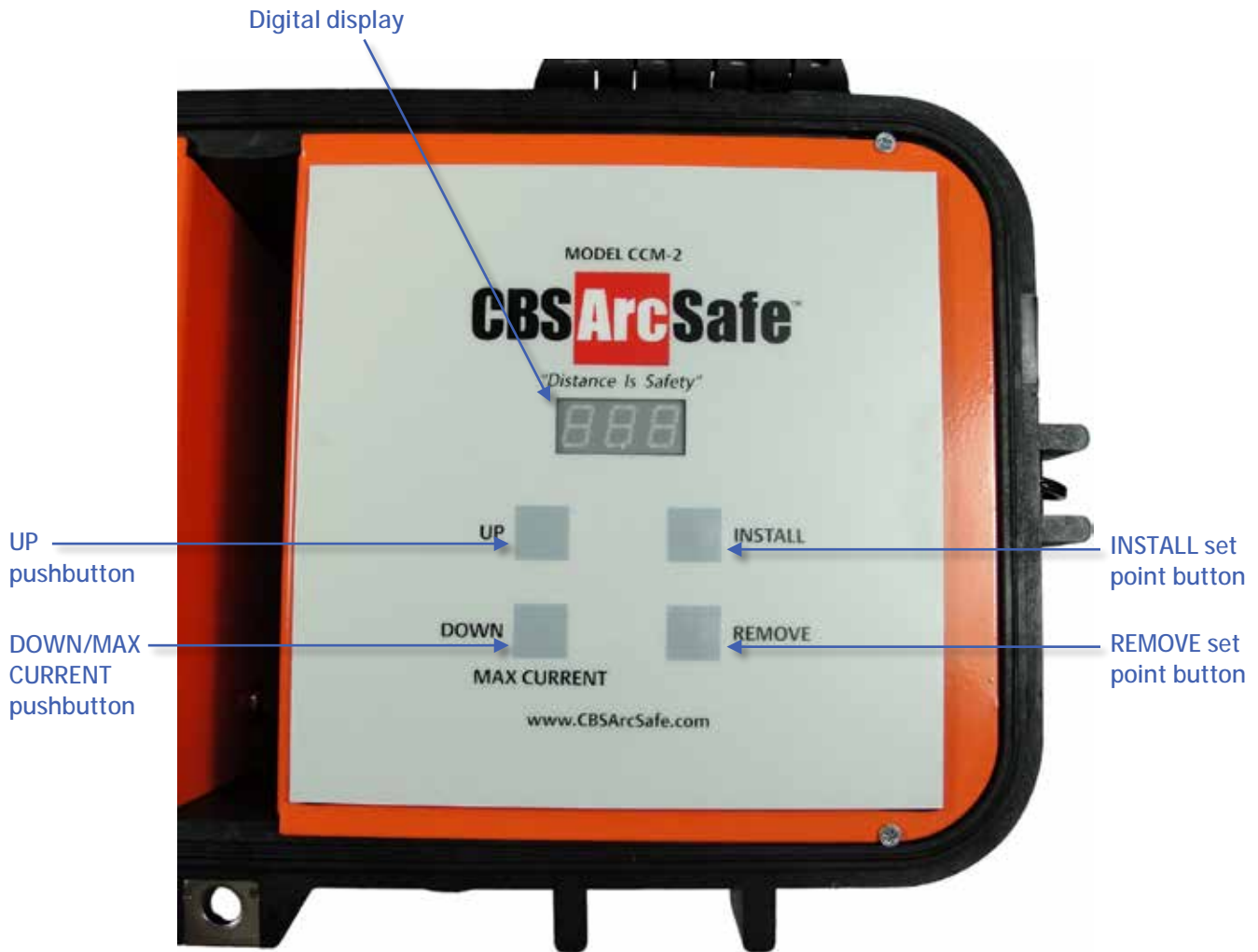
Figure 5-3: RSO Control Panel Components
