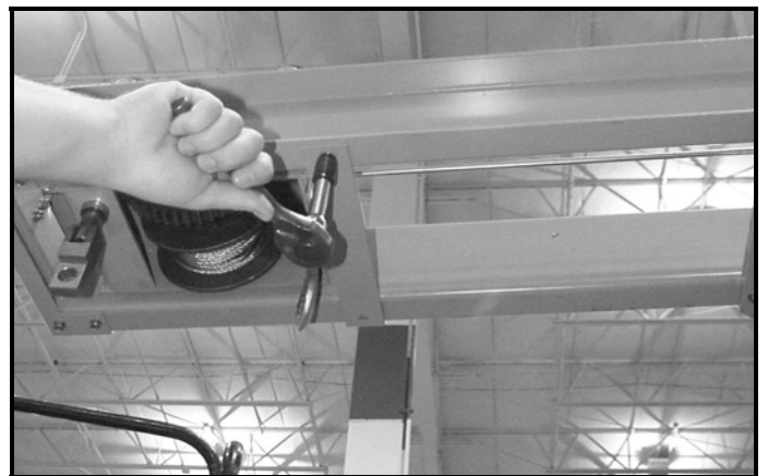
Fig. 4-25. Removing the bracket locking the hoist dolly
