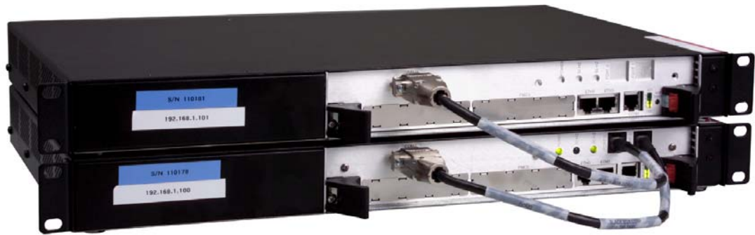
Figure 1-15 Redundant CPUs with synch clock connection
