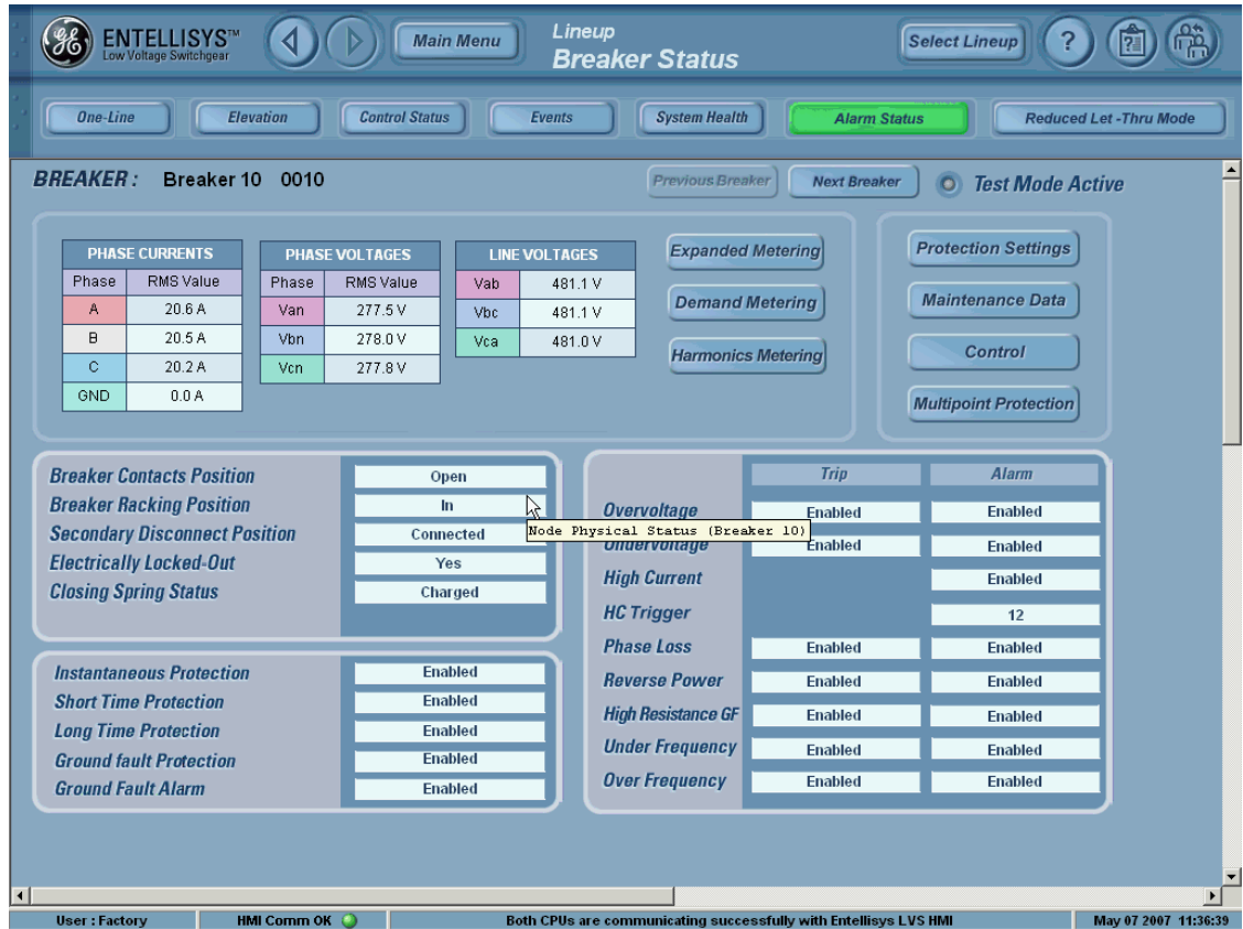
Figure 3-18 Breaker Status screen
