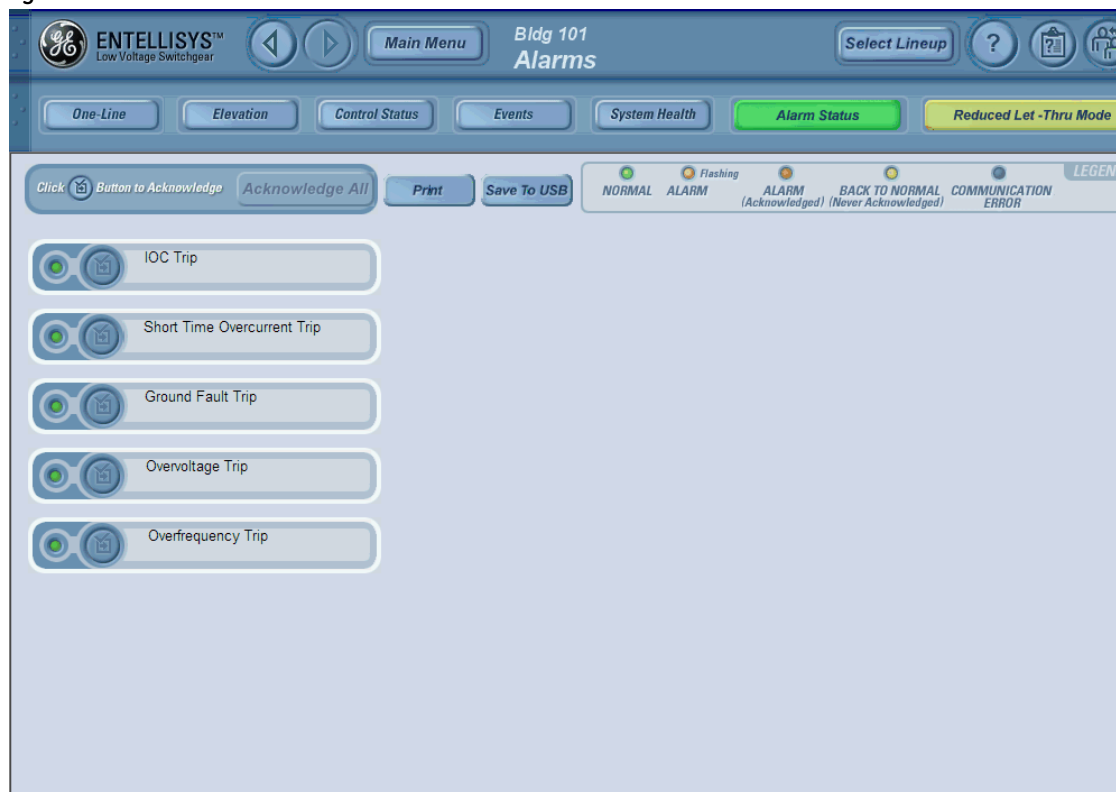
Figure 3-33 Alarm Status screen
