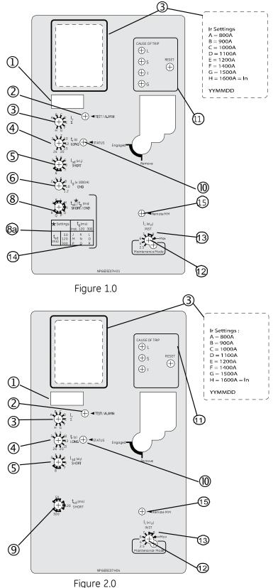
7-1 . Test Port - a test port is built into each trip unit to allow use of a functional test kit. The test kit performs a test of the Long Delay, Short Delay, and Ground Fault functions.
