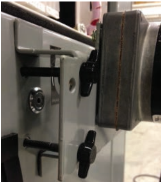
Figure 4a: Fastening motor on door.
