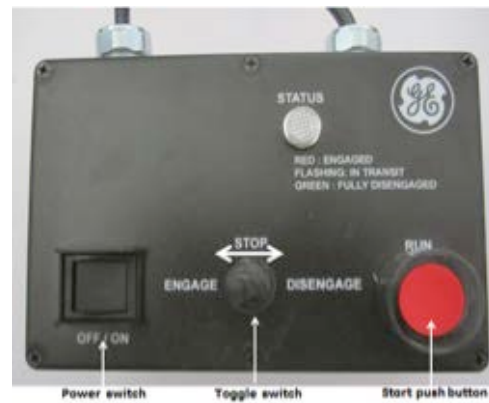
Figure 6a. Pendant operation details
