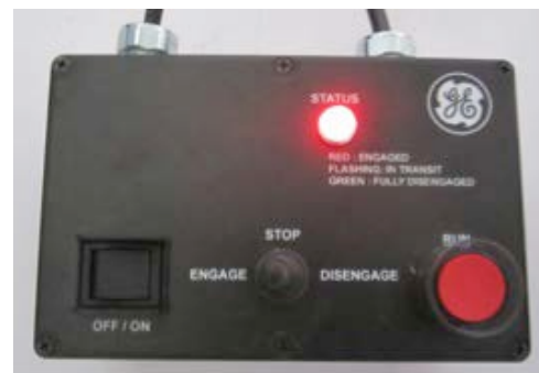
Figure 6b. Controller showing ENGAGED condition
