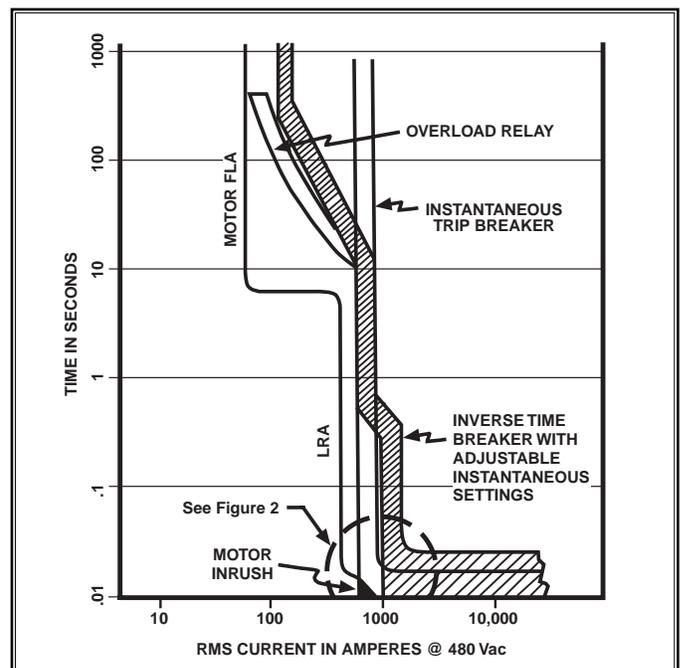
Fig. 1 is a time versus rms current plot showing a 150A frame, 125A rating, inverse time molded case circuit breaker with adjustable instantaneous trip as part of a combination controller for a 60 horsepower energy efficient motor which draws 65.3 full load amperes at 460Vac. The inverse time cir-
