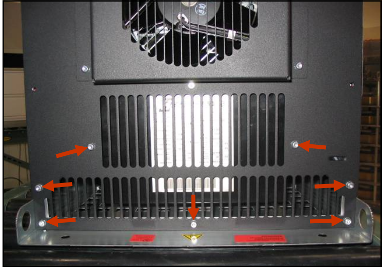
Figure 4. Screws to be removed from top of drive
