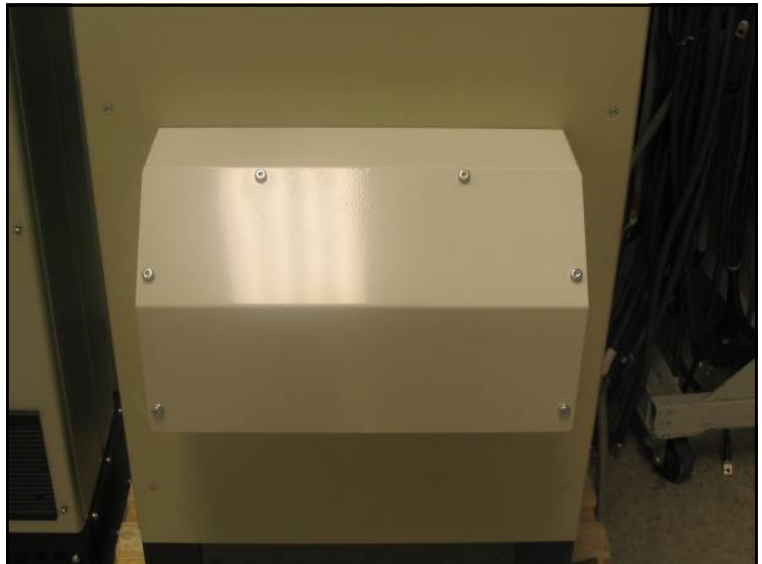
Figure 21. Lower deflector assembly installed
