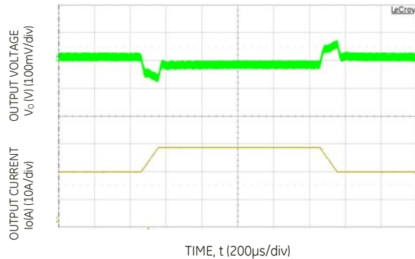
Figure 4. Transient Response to 0.1A/μs Dynamic Load Change from 50% to 75% to 50% of full load, Vin=48V
