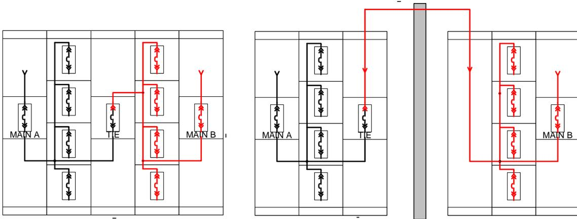
Looking at the above scenarios, the customer went to the extra trouble and expense to separate the two sides of the service board. However, even if the source to Main A was de-energized as depicted there is still live bus in side A. The technician in this case cannot work on a de-energized lineup and must still be concerned about shock hazards and must still wear the appropriate PPE for the present hazard risk category.
