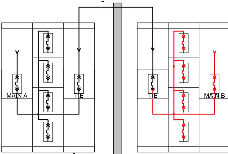
By separating the two sources and by employing double tie breakers, each side of the board can be truly de-energized for maintenance and an operator can remove himself from the dangers of shock hazards and arc flash.
