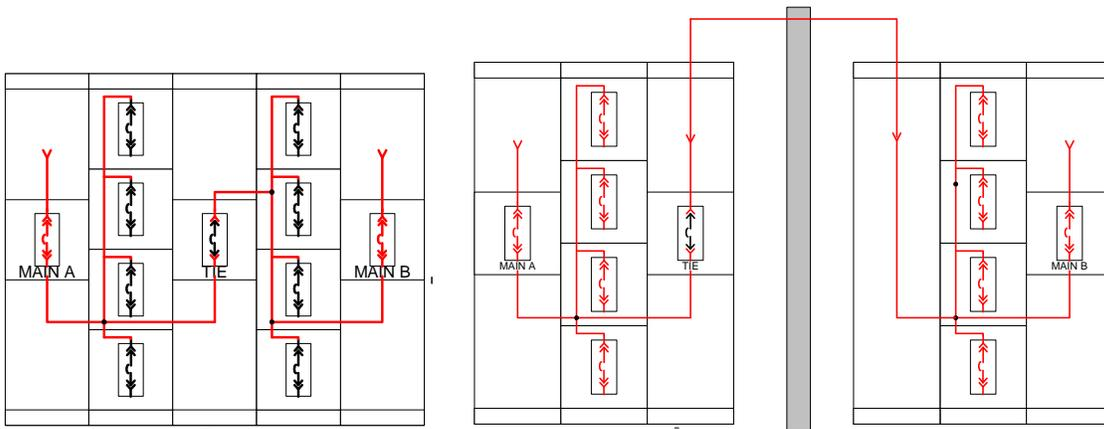
The above scenarios have live bus in each and every section during normal operation with tie open and both mains closed.
