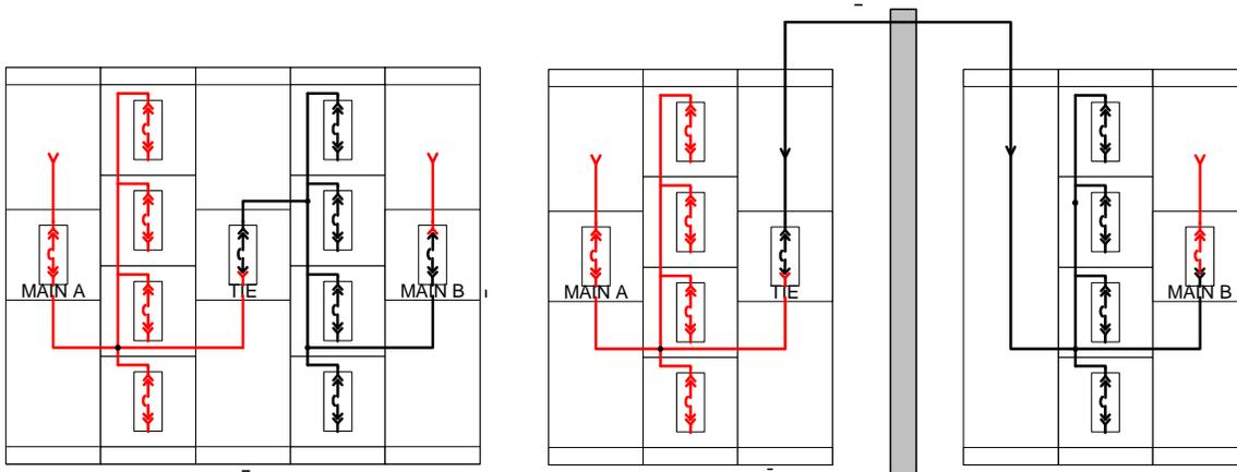
The maintenance personnel should clearly understand that the line side of source B breaker is live bus while everything between the load side of Main B and the Tie is de-energized. Prudent maintenance technicians will even go the extra step and remove the source to the line side of Main B so that for lineup 2, the entire board is dead and they can safely work on de-energized equipment.
