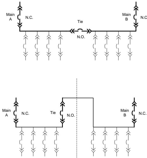
The following diagrams depict the above distribution one-lines as an elevation in equipment. The red bussing indicates which bussing segments would be energized in normal operation. Normal operation defined as Normally open tie breaker with Normally Closed incoming breaker.
