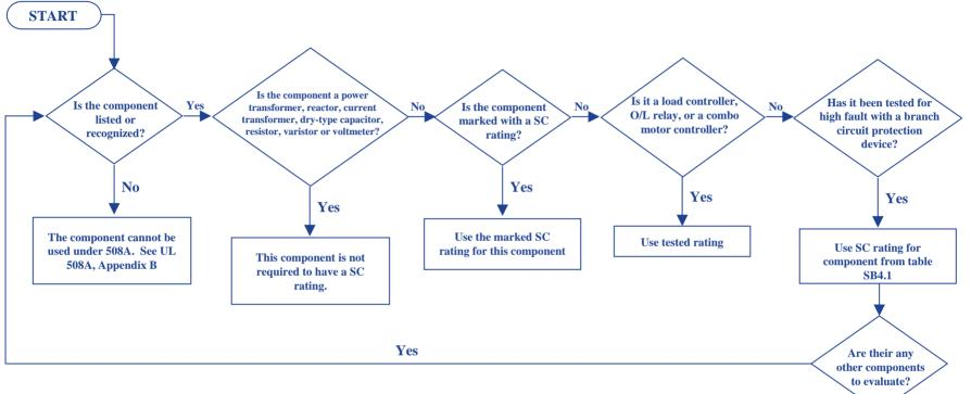
Compare the SC rating of the lowest rated component with the SC rating of the branch circuit protection device. The smaller of the two ratings is the SC rating for the line side of the PCPD. Proceed to SB4.3
