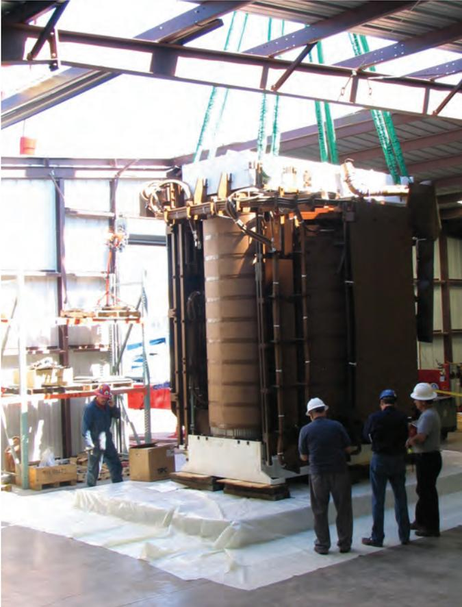
Once the transformer is inside and ready for disassembly, all access is through a man door where particulate contamination is controlled and where all individuals entering the main building are required to wear new, clean foot protection.
