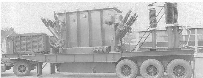
1966 30 MVA GE Mobile Substation as received.
