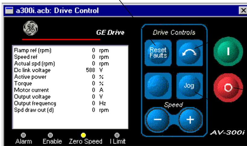
Click here to toggle the direction of the drive (reverse request). The selected direction is shown with an icon
