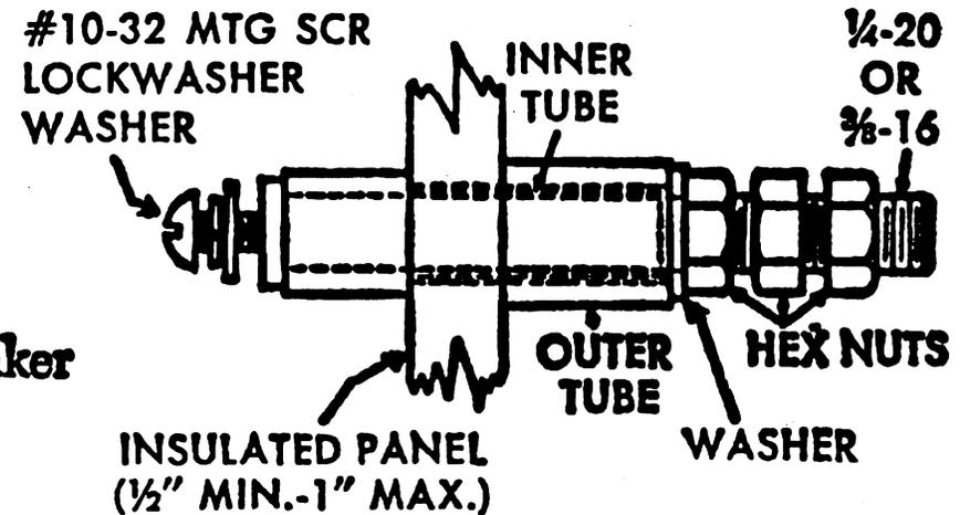
View through panel showing typical assembly of parts
