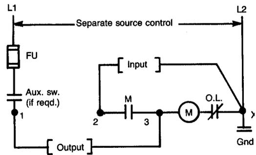
**Fig. 7. INPUT and OUTPUT Connections for Separate-Source Control**
